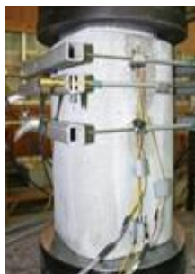
Fig. 10 Test setup of strengthen column
