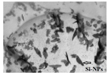
Fig. 1. Overall view of Si-NPs under TEM
