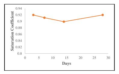
Fig.13. Effect of Mechanical Mixing on Saturation Coefficient at 5% Waste Addition
