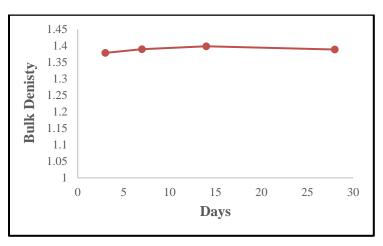
Fig.9. Effect of Mechanical Mixing on Bulk Density at 5% Waste Addition
