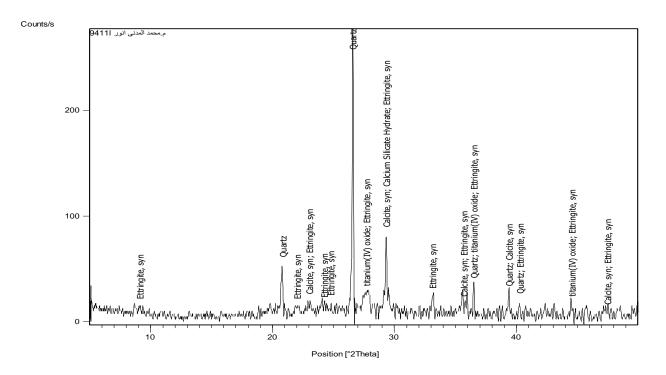
Fig.7. XRD Pattern of a Specimen after 14 Days
