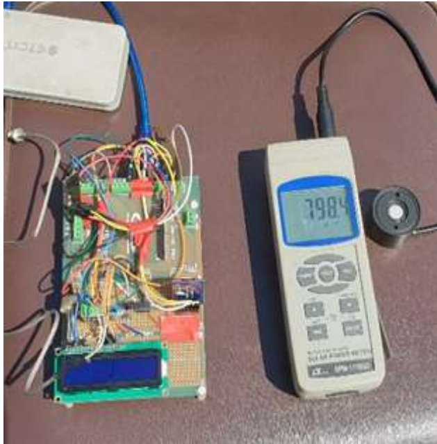
Figure 14: The calibration and testing of LDR SENSOR using a solar meter.
