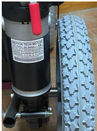
Figure 13: The used DC motor
