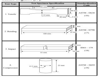
Fig.7 molds of tests
