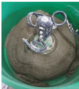
a) Mixing of GP mortar
