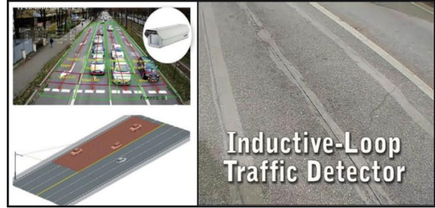
Figure 4: Example of the queue length detection methods; the right is the inductive loop and the left is CCTV Camera
