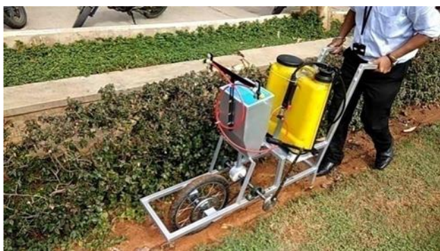
Fig. 9. A mechanically operated pesticide sprayer and fertilizer dispenser (Akshaya et al., 2017).
