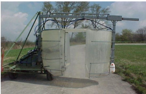
Fig. 2. A recycling tunnel sprayer (Molari et al., 2005).
