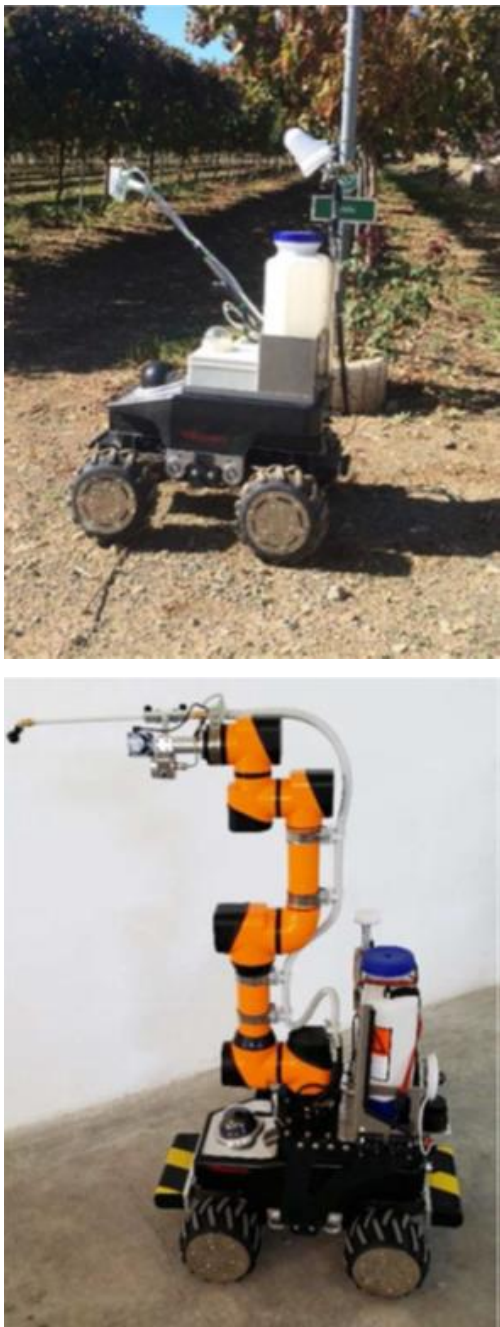
Fig. 6. Semi-autonomous agricultural vineyard sprayer (Adamides et al., 2017).
