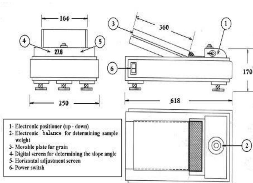
Figure (1): Elevation, plan and side view of the digital equipment used for measuring the friction coefficient
