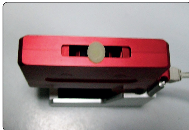
Fig. (2): Photograph of Zehntner glossmeter
