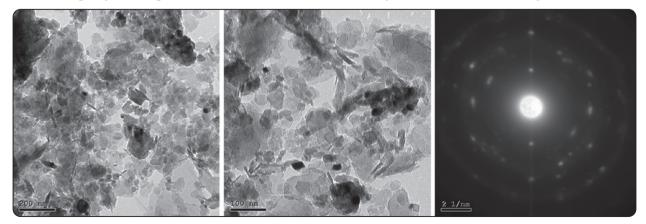
Fig. (1) TEM images showing coral calcium nanoparticles
