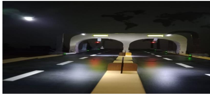
Figure (3): Smart lighting by LDR & PIR sensors in the prototype in dark times
