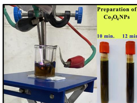
Figure (2): Synthesis of \text{Co}_3\text{O}_4 NPs by Atmospheric Plasma Jet at 10 and 12 minutes.
