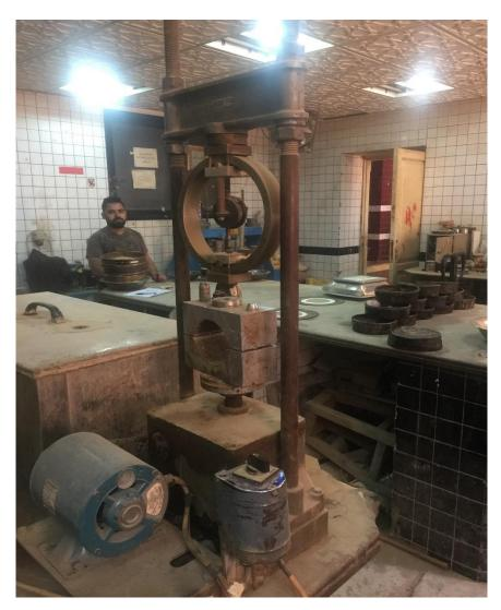
Fig 2: Marshal stability- flow test
