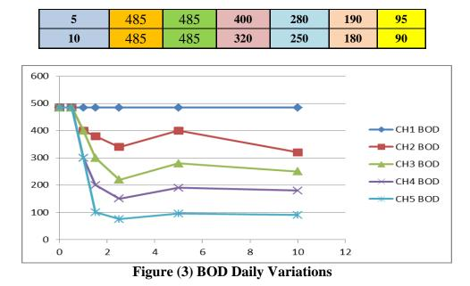
It was found that, BOD decreased with plastic media in general from 485mg/l to 340-75 mg/l according to the length of the media and the distance after it with removal ratio from 29.8% to84.5%. For the water velocity increase during its passage through the media voids that helps air dissolving in water and encourage the attached growth bio action to take place inside the media
