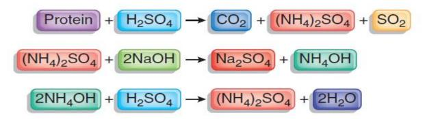
Figure 2. Kjeldahl method, a universally used quantitative method for assessing protein content in food.
