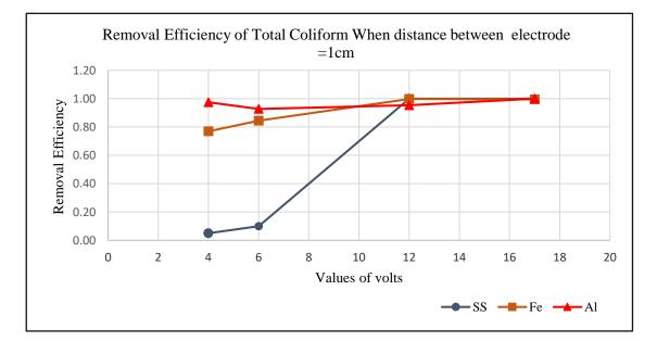
Fig.7. The efficiency of removal Total coliform with different types of electrodes when d =1cm
