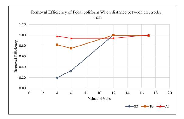
Fig.8. Removal Efficiency of Fecal Coliform with different types of electrodes when d=1cm
