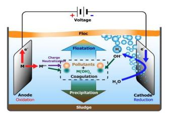
Fig.1. Electrocoagulation Concept. [8]
