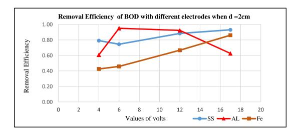
Fig.10. Removal Efficiency of BOD with different types of electrodes when d=2cm
