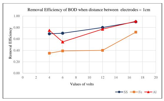
**Fig.5**. Removal Efficiency of BOD with different types of electrodes when d = 1cm
