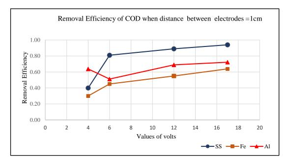
Fig.6. Removal Efficiency of COD with different types of electrodes when d=1cm
