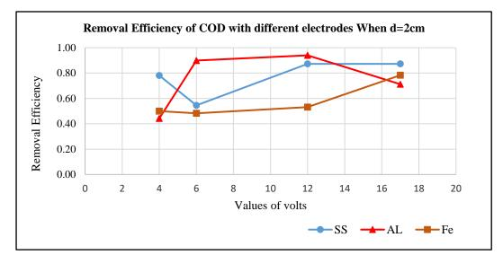
Fig.11. Removal Efficiency of COD with different types of electrodes when d=2cm
