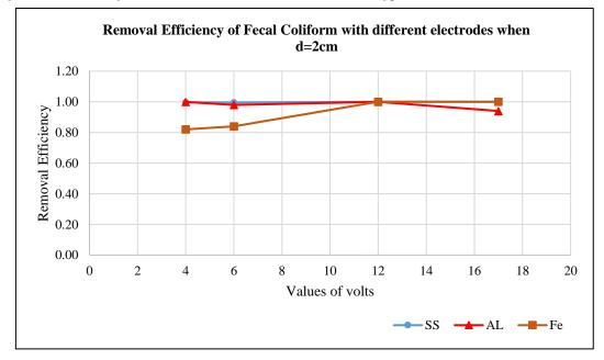
Fig.13. The efficiency of removal of fecal coliform with different types of electrodes when d=2cm
