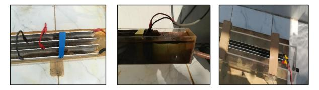
a) Aluminum b) Iron c) Stainless Steel **Fig.4**. Different types of electrodes a) aluminum, b) Iron, c) Stainless steel with the spacing between electrodes 1cm
