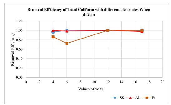
Fig.12. The efficiency of removal of total coliform with different types of electrodes when d=2cm
