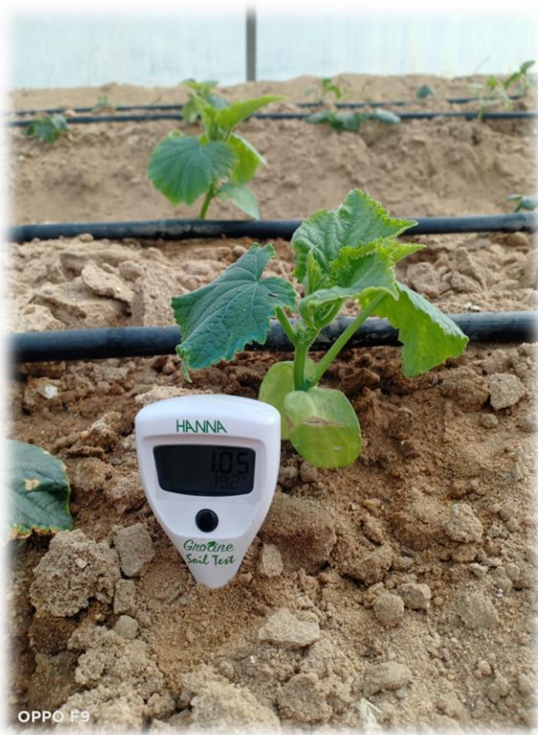
Measurement of the conductivity and temperature of soil which is used in smart irrigation scheduling (left photo), saving irrigation water by using plastic mulch which reduces evapotranspiration
