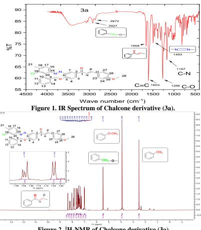
Figure 2. <sup>1</sup>H-NMR of Chalcone derivative (3a).
