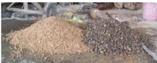
(a) Before mixing recycled to natural aggregate
