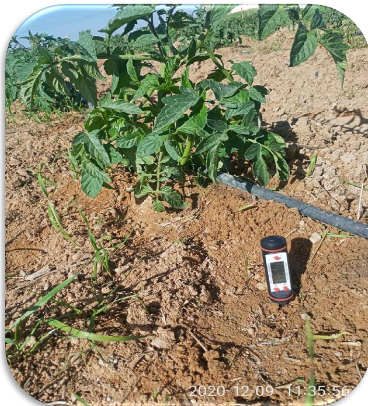
Monitoring some of soil properties such as EC, pH and temperature
