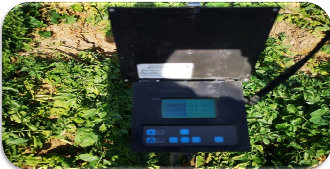
Automatic board used irrigation water scheduling
