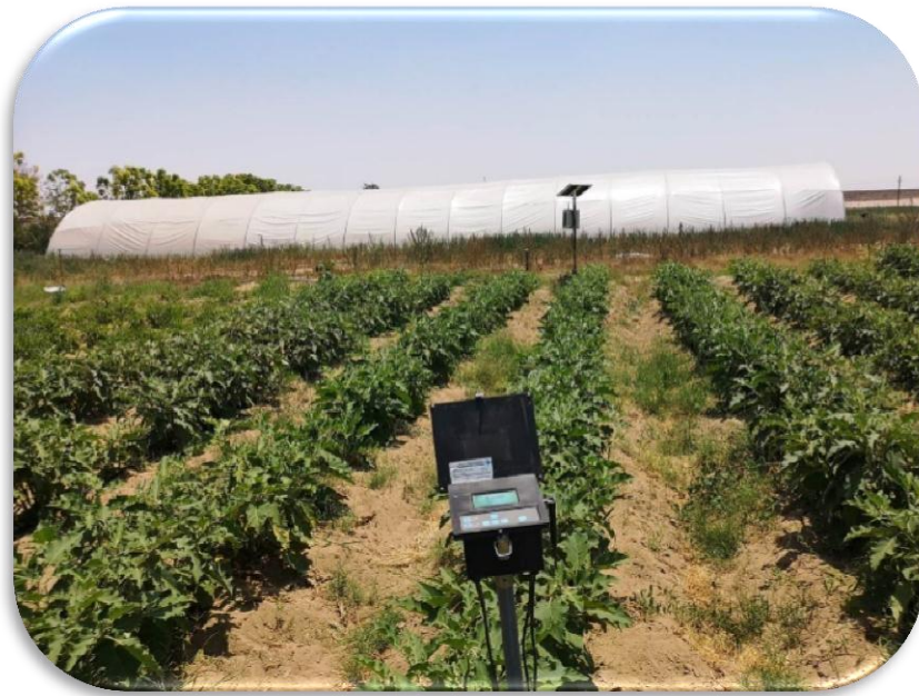
Monitoring station of soil moisture content and soil temperature at different depth by sensors at plant development stage
