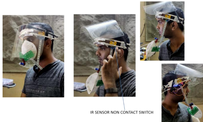
Figure 16. Hardware Prototype of Smart Mask and face shield
