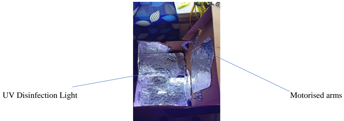
Figure4. Hardware prototype of UV disinfection box
