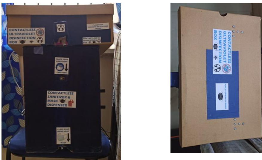
Figure 7. Hardware prototype of Smart portable covid clinic equipped with contactless sanitizer, mask and UV disinfection box
