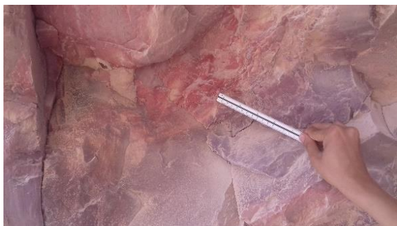
Fig. (10): Ferrugination of kaolinite in top part of level D lens along contact with the overlying sandstone bed, at Shushet Abu El-Nimran
