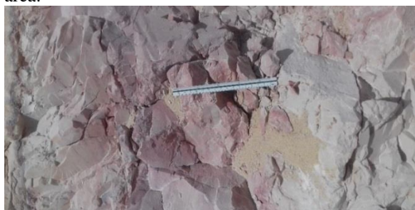
Fig. (14): Ferruginated kaolinite at the middle part of level D kaolinitic clay lens, at Salia area
