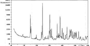
Fig (2): X-ray diffractoagram of calcium oxalate monohydrate crystals. Specific surface area:
