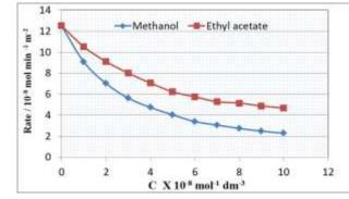
Fig (5): Plot of the rate of crystal growth of COM crystal against [methanol and ethyl acetate extracts] of *Anastatica hierochuntica* L at  $\sigma = 0.4$ , t = 37 °C and I = 0.15 mol dm-3.
