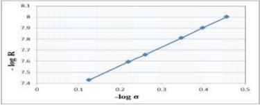
Fig (4); Plots of –log R against –log  $\sigma$  for crystal growth of calcium oxalate monohydrate crystals at 37  $^\circ C$
