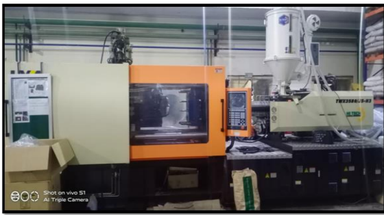
Figure 2 Injection Moulding Machine (Tederic 360)
