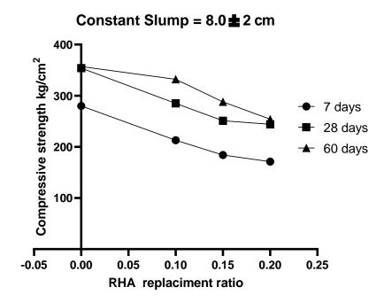
Figure 2: Effect of RHA on concrete compressive strength without using plasticizer
