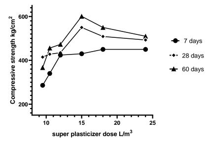
Figure 4: Effect of different doses of superplasticizer on concrete compressive strength with an optimum RHA replacement ratio of 10%
