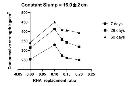
Figure 3: Effect of different RHA content on concrete compressive strength with plasticizer
