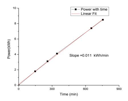
Figure 9. Relation between the power consumption and time.
