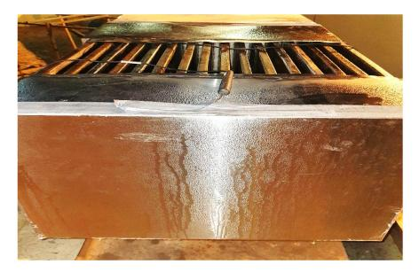
Figure 7. Photo of condensation of water on the surface of the attachment.
