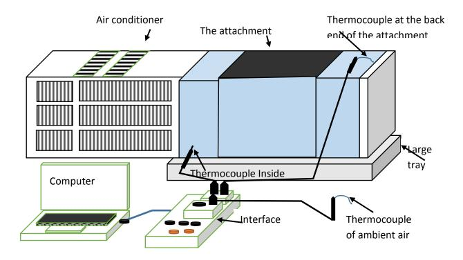
Figure 3. Schematic diagram of the system components and the experimental setup.
