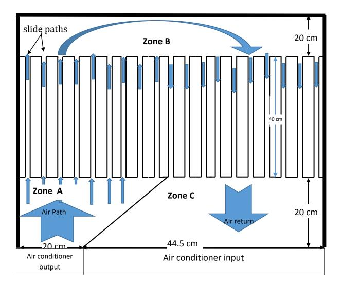
Figure 1. Schematic diagram of the attachment.
