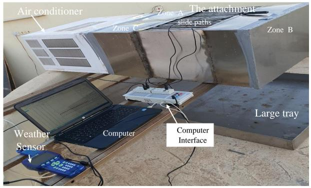
Figure 4. Photo of the complete system during the measurements.
