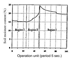
Fig. (10): Moisture response transient using ON-OFF controller.
