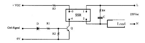
Fig 1: The solid-state relays (SSR) circuit diagram.
