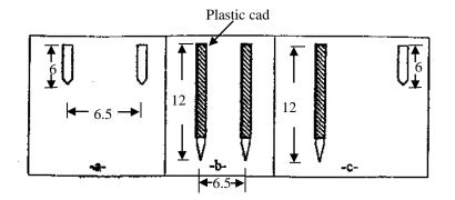
Fig. 4: Different shapes and arrangements of the two-electrode sensor.
