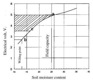
Fig. 7-B: Calibration of the two-electrode sensors.
