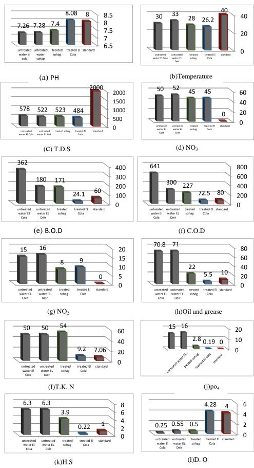
Figure 1. Assessment of untreated, treated sewage physicochemical parameters and their criteria.
