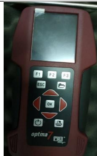
Figure 4 exhaust gas analyzer optima 7
