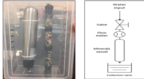
Figure 7: (A) Water Addition filter and UV system (B) Configuration of mineral addition test
