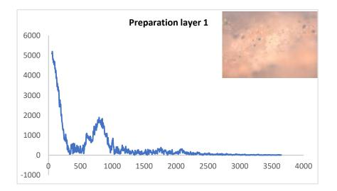
Fig 6. The sample of preparation layer showed the presence of calcite and clay minerals and a percentage of animal glue **Black pigment**
