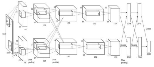
Fig 9. the network structure of Alex Net
