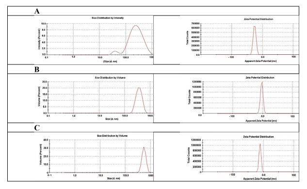
Figure 1: Z average size and Zeta potential of cinnamon (A) ginger (B), and orange (C) nano-emulsion of the tested plant oils.
