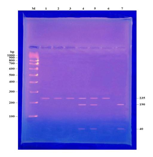
**Figure S 1:** The ethidium bromide-stained agarose gel electrophoresis image demonstrates the restriction enzyme digestion of the PCR result (Rsal) in which there was the analysis of the HNF1A rs55783344 CT gene polymorphism in CAD patients . DNA size marker (100bp) ladder. Lanes (1,2,3,6): CC genotype showing the presence of one band 235 bp. Lanes (7): TT genotype showing the presence of two bands 190+40 bp. Lanes (4,5): CT genotype showing the presence of three bands 235+190+40 bp.
