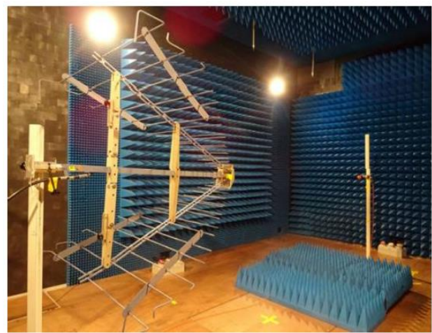
Figure 15. Test setup with single LPDA, originally from reference [120]
