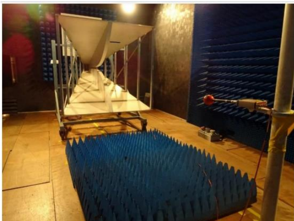
Figure 16. Test setup with Ext-DRGH originally from reference [120]
