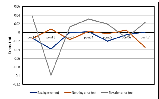
Fig. 17: ICPS Errors for DG/reference aligning technique
