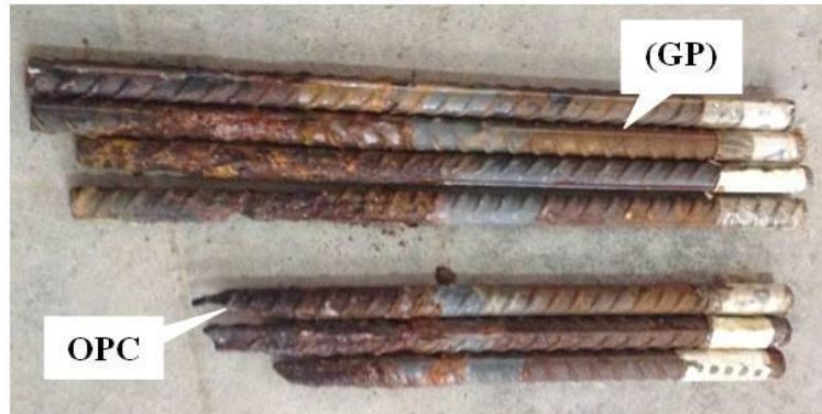
Fig. 18: Retrieved rebars after accelerated corrosion testing
