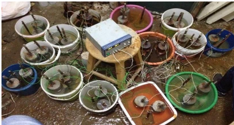
Fig. 2: Accelerated corrosion test setup
