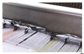
Fig (11) Weaving Head - Filling insertion. (7)
