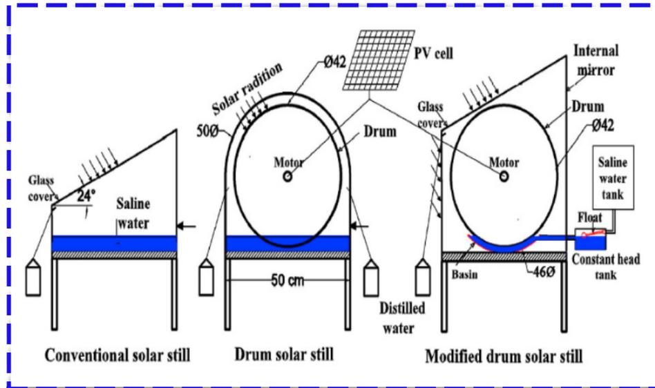
Fig. 16. A lay-out of modified drum distiller [36].
