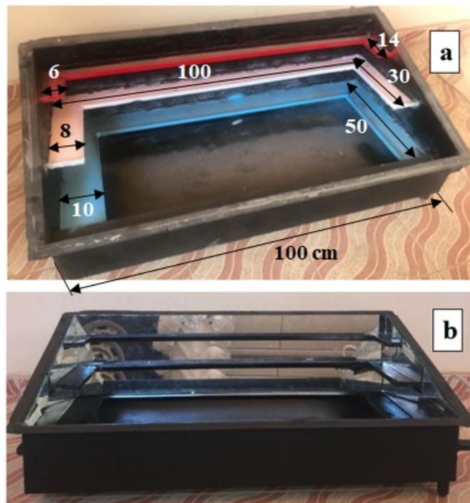
Fig. 6. Trays solar still, (a) Trays before applying black paint (b) inside mirrors [8].
