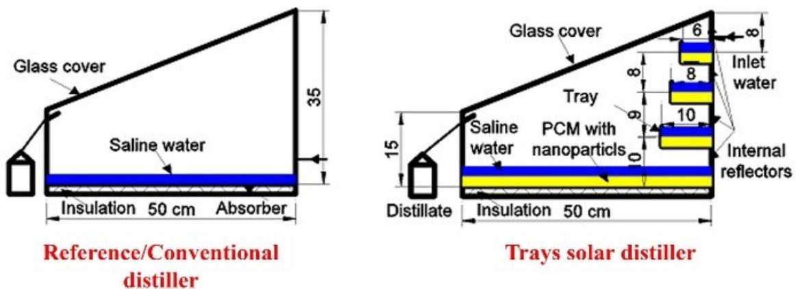
Fig. 7. Cross-sectional view of trays with PCM [29].
