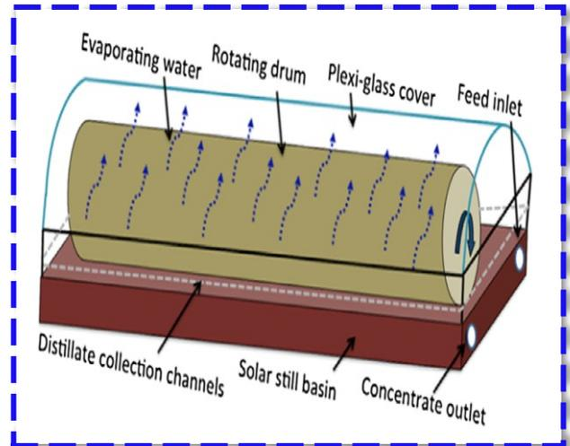
Fig. 13. A graph of a rotary drum inside an adjusted distiller [33].
