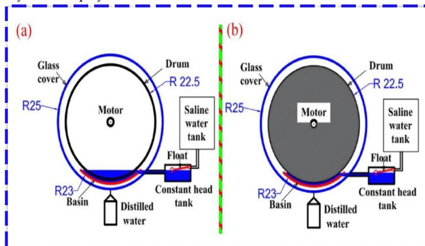
Fig. 17. An illustration of the tubular SSs that were investigated shows (a) open-ended drum and (b) closed-ended drum. [37].
