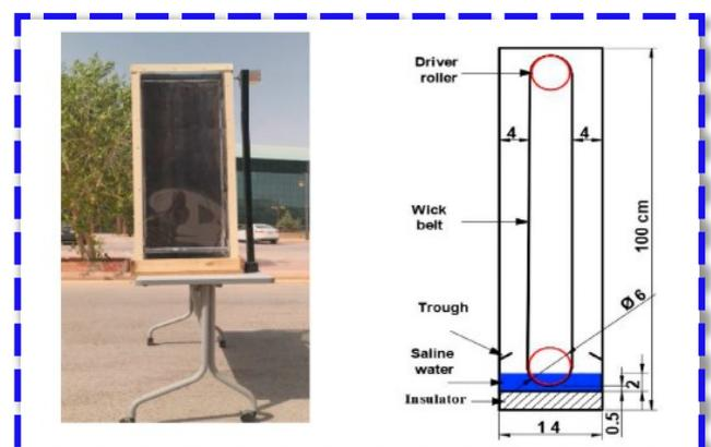
Fig. 23. A vertical distiller's design and graph with a rotating wick belt [44].
