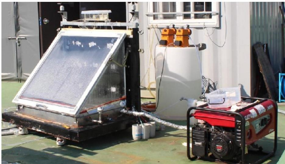
Fig. 4. Test setup for hybrid multi-effect diffusion still experiments [28].
