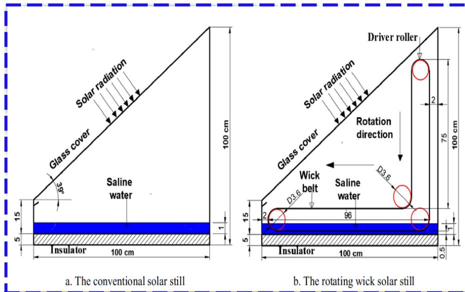
Fig. 21. The spinning wick distiller and conventional distiller designs [41]
