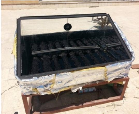
Fig. 11. Image of the corrugated wick still with the vacuum and mirrors [31].
