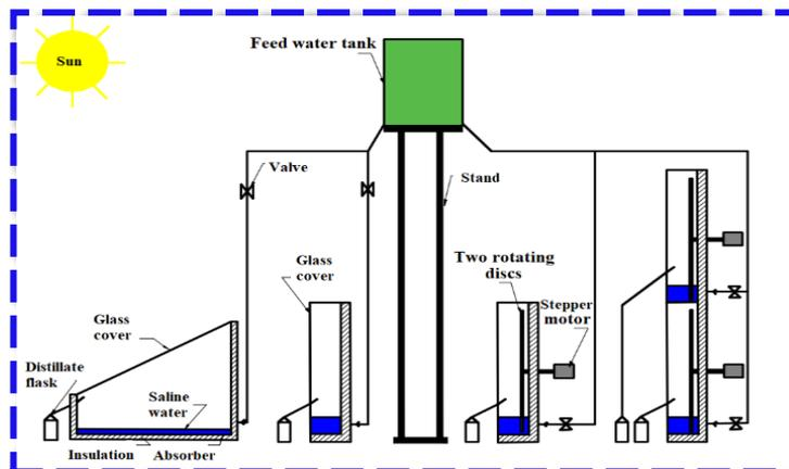
Fig. 19. Diagrammatic representation of the rotating discs addition to the vertical solar still [39].
