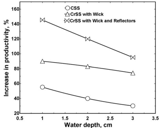
Fig. 9. Productivity increases for conventional still (CSS) and corrugated still (CrSS) [30].
