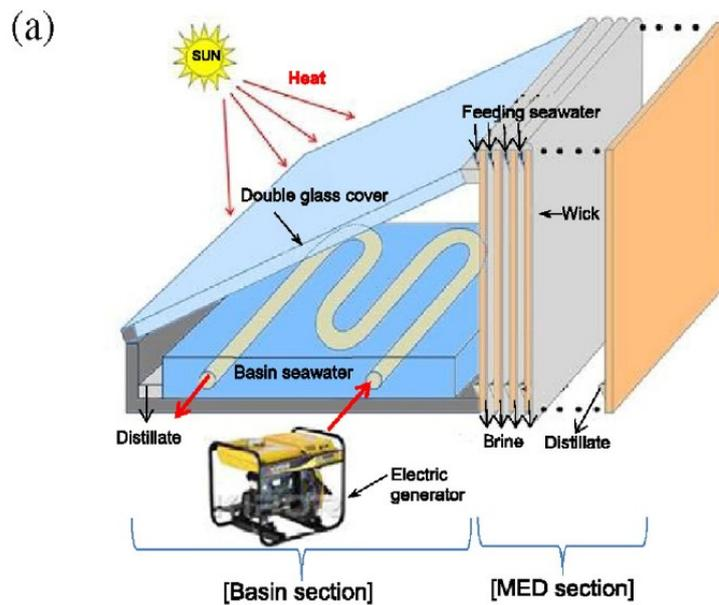
Fig. 3. Hybrid multi-effect diffusion still's schematic [28].
