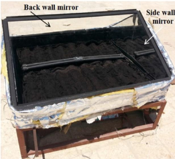
Fig. 8. Corrugated absorber solar still with mirrors and wick [30].
