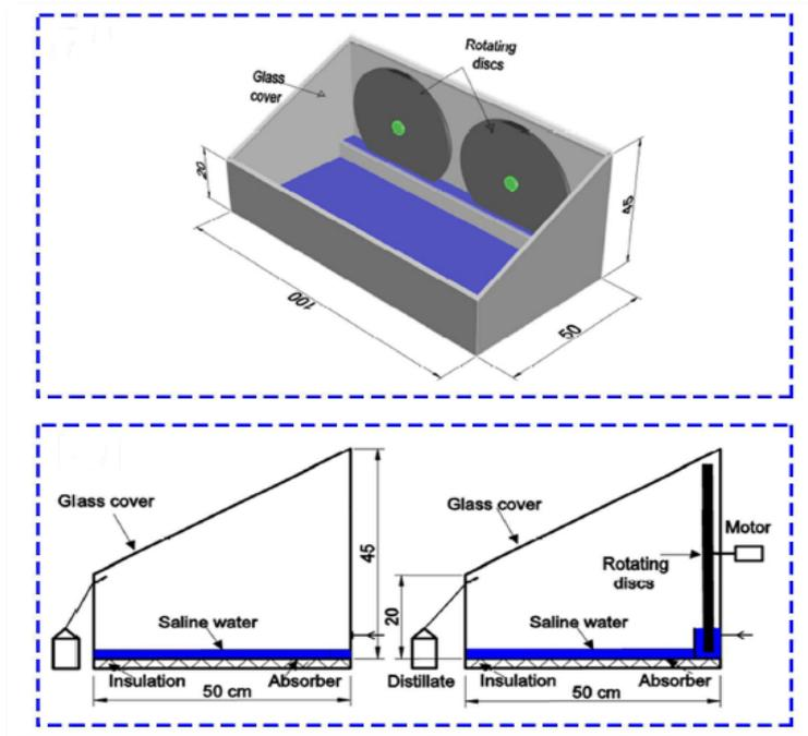
Fig. 18. Schematic illustration of the rotating disc solar still [38].
