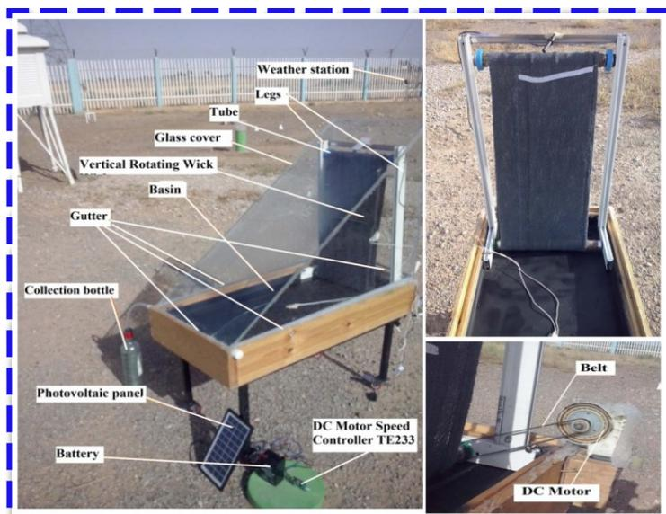
Fig. 20. A picture of the test rig for experiments [40].
