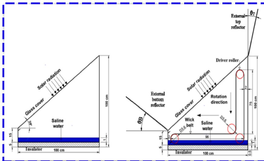
Fig. 22. The configuration of the spinning and traditional wick distillers [43].
