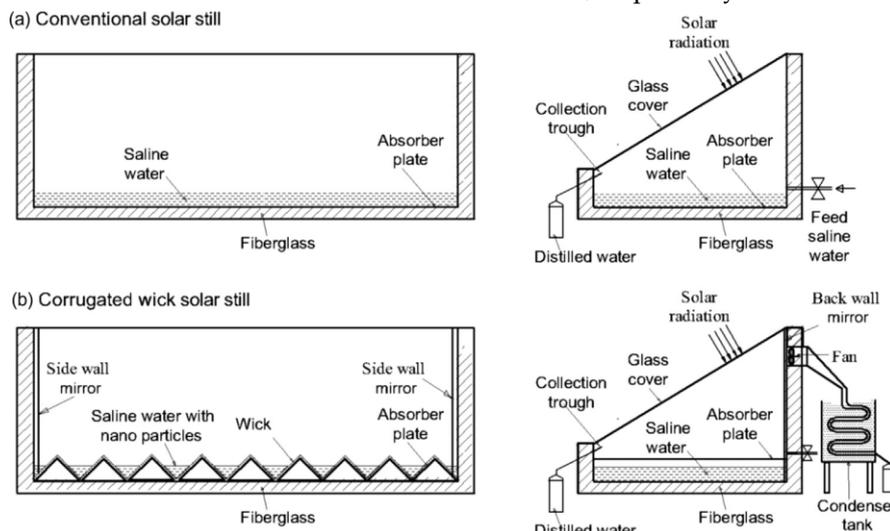
Fig. 10. Schematic of solar stills [31].
