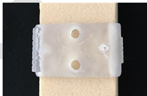
Fig. (2): Final 3D printed surgical guide perfectly fitting on the test block.
