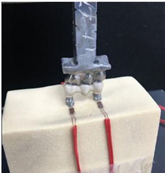
Fig. (4): Vertical occlusal loading of the test specimen FPD framework seated into its position with the previously fabricated occlusal loading device attached to the Universal testing machine.
