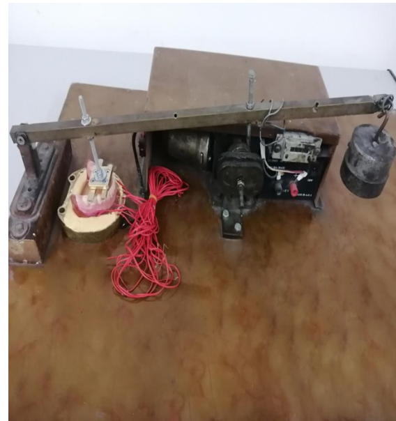
Figure 6: Application of cyclic loading of 10N.
