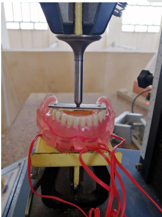
Figure 5: Application of vertical load of 60 N.
