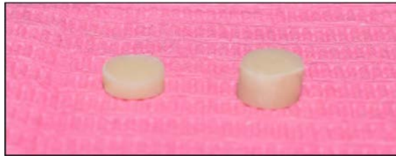
Figure 2: composite discs 2mm and 4 mm in thickness.
