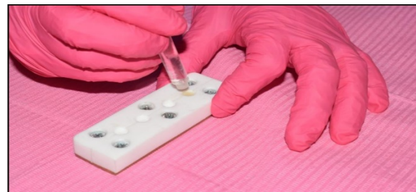
Figure 1: Teflon molds with dimensions 6 mm in diameter 2mm or 4mm in thickness
