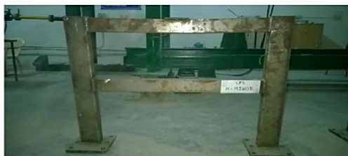
failure in minor axis
