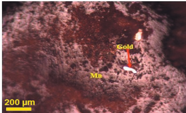
Fig. 26: Reflected light photomicrograph showing very fine grain of gold enclosed in manganese (pyrolusite) , XRL
