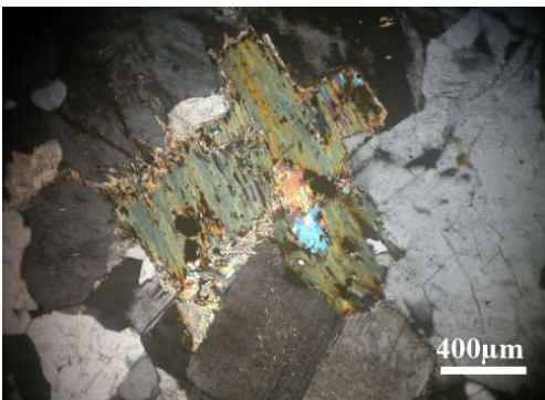
Fig. 31: Highly chloritized biotite with relicts of muscovite, Gabal Kab Amiri monzogranites, XPL
