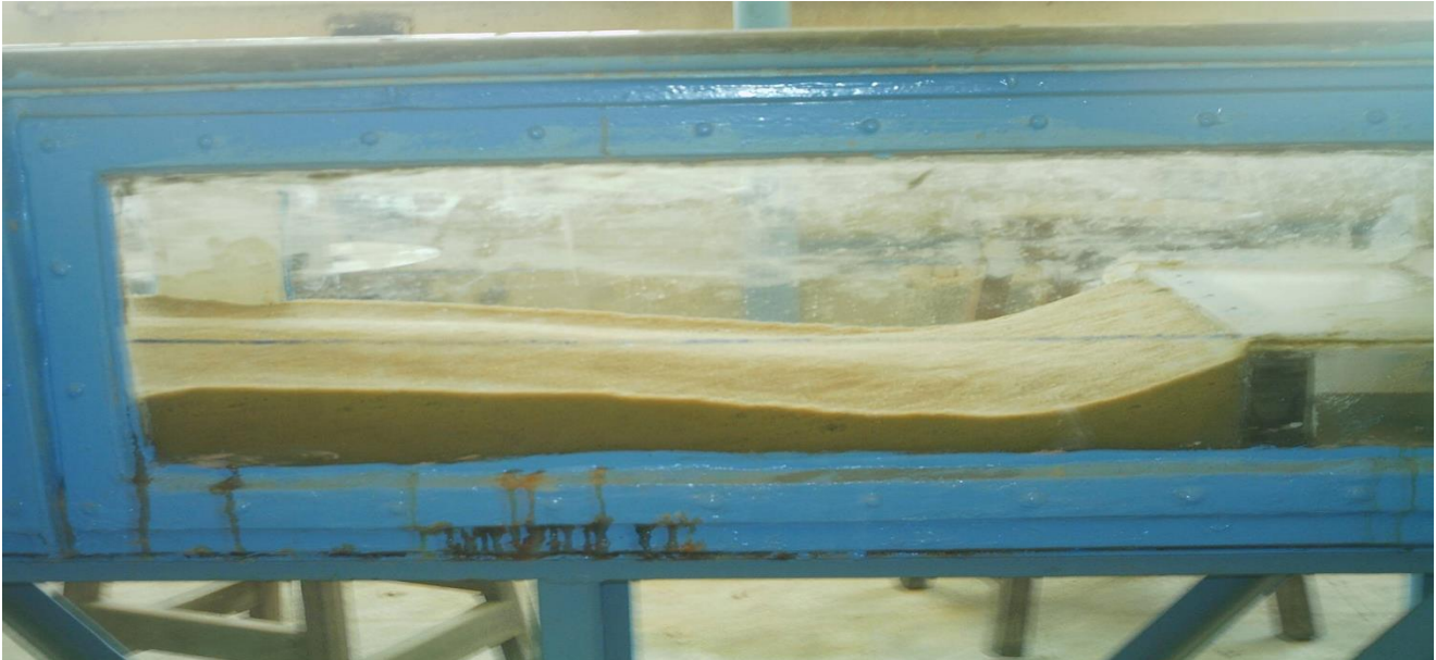
Photo (3) Scour Downstream apron
