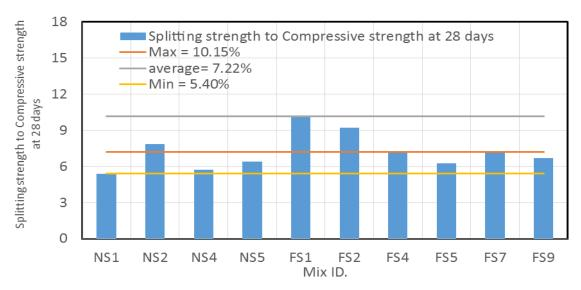
Fig. 9: The ratio between splitting strength to Compressive strength (SCR) at 28 days.
