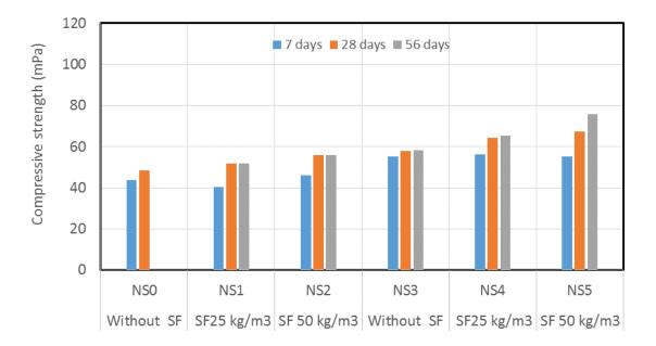
Fig. 4: The compressive strength for mixes NS0 to NS5.
