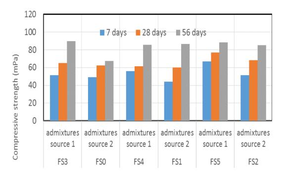
Fig. 7: The effect of admixtures source on compressive strength
