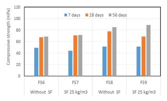
Fig. 6: the compressive strength for mixes FS6 to FS9.
