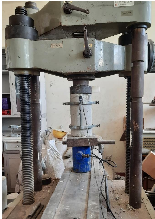
Figure 4: Testing of concrete compressive strength of filling in CFT columns in order to calculate modulus of elasticity E_c
